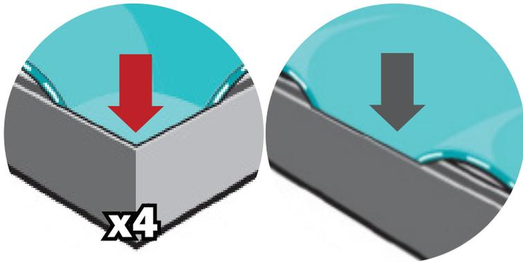
Fit graphic into corners, then "tap" into rest of frame channel.
