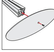
**Base Plate & Extrusion Connection**
