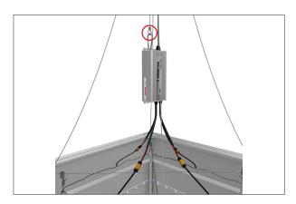
**Step 14:** Test lights if possible to make sure it has been wired properly.
