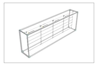
**Step 8:** Assemble center support brace by pushing and pulling together.
